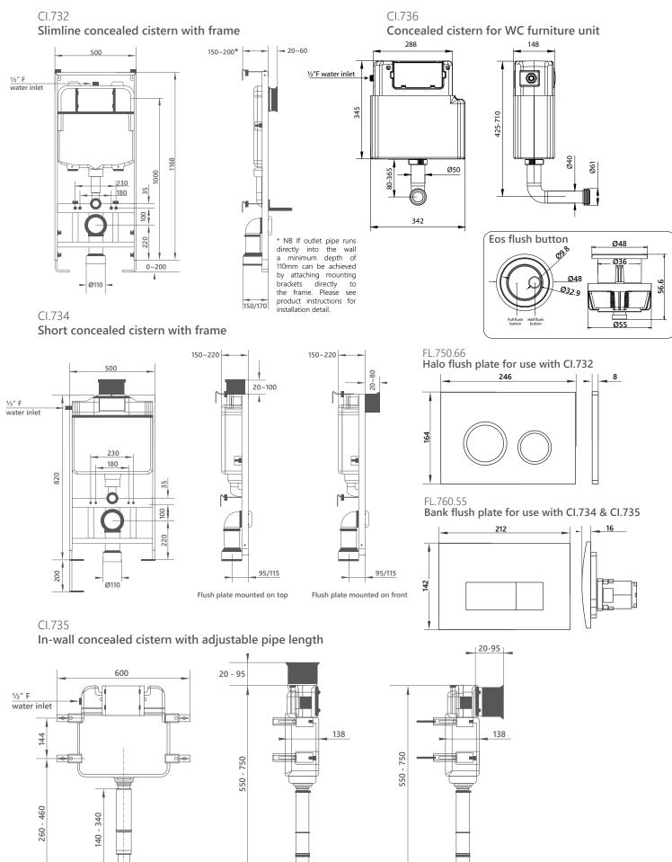
Flush plate mounted on top
